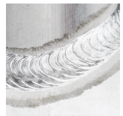
Without SFI (spatter-free ignition)
